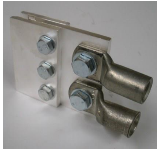
Temporary cable connection onto 6.35mm busbars (approx. 2000A)
