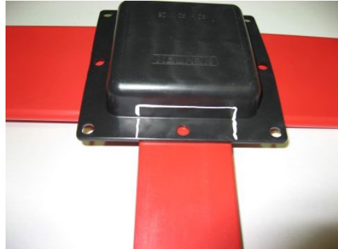
Mark the areas to be cut (A white ink marker is recommended)
