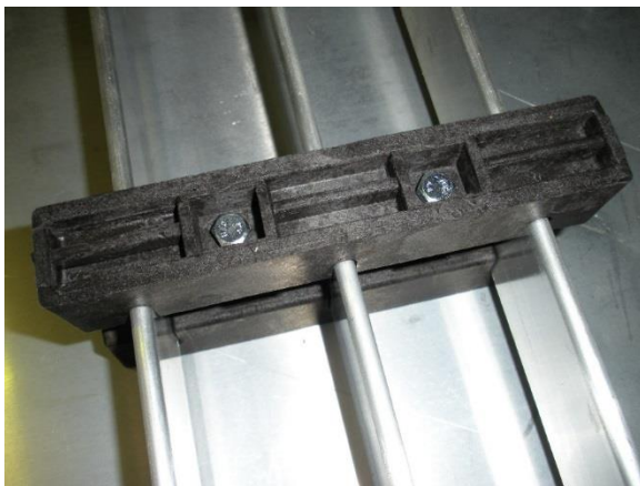
M6 bolts (or nuts) inside of pocket
